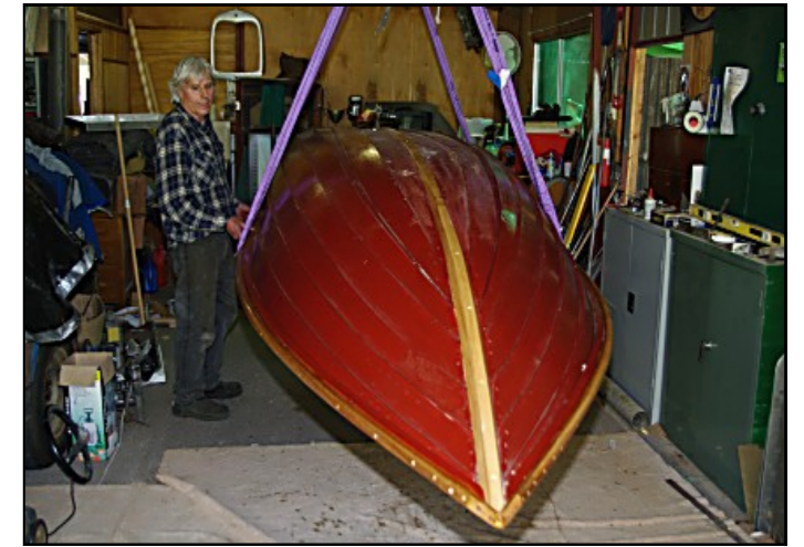
Straps now ready to come off after settling the hull on trestles
