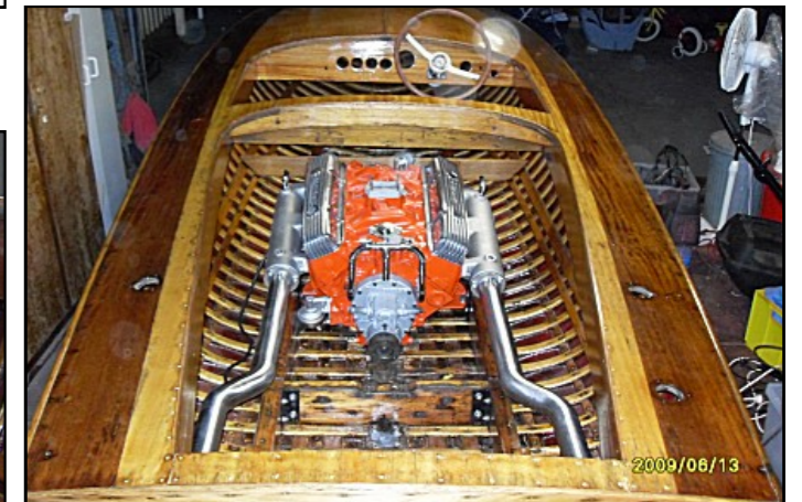
Motor back in and new exhausts. Had to buy new exhaust manifolds as the old ones were corroded and they were different, so new stainless steel exhausts. Thank-you Greg Nelson!
