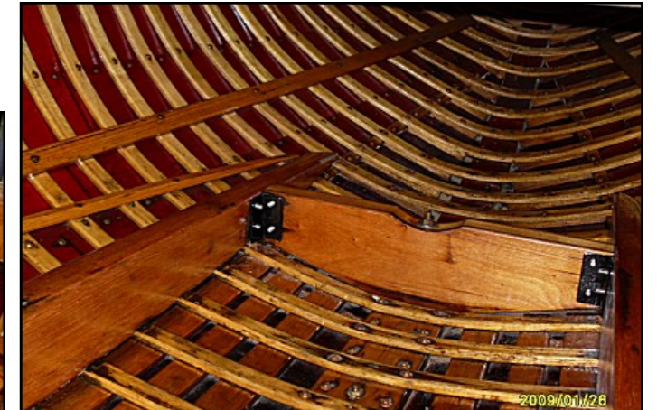
Inside the hull again after varnishing. The deck was also sanded back, stained and revarnished, and although not perfect, it did come up a lot better than I thought it would.
