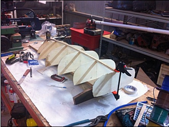
Construction detail is quite fine and accurate to the real boat, as can be seen by the deck frames, details that will be covered later by the deck.
