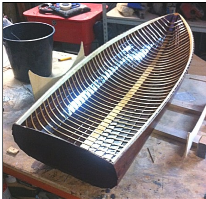
Construction detail is quite fine and accurate to the real boat, as can be seen by the deck frames, details that will be covered later by the deck.
