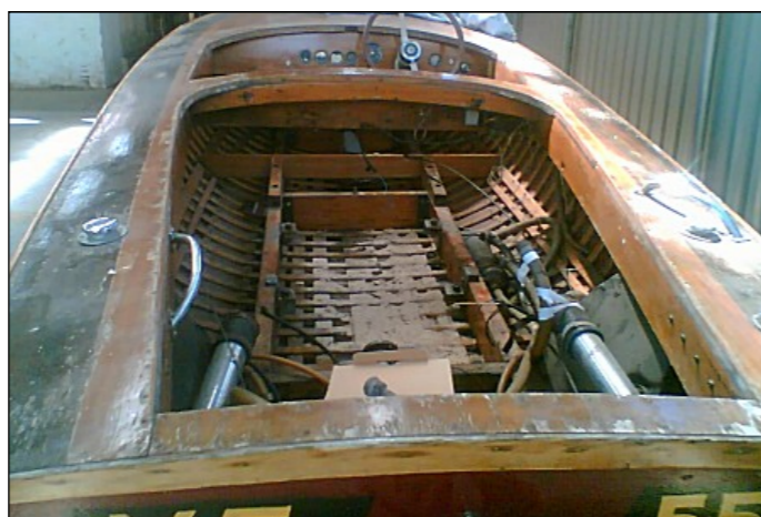
Motor out and sawdust in - to try and soak up some oil
