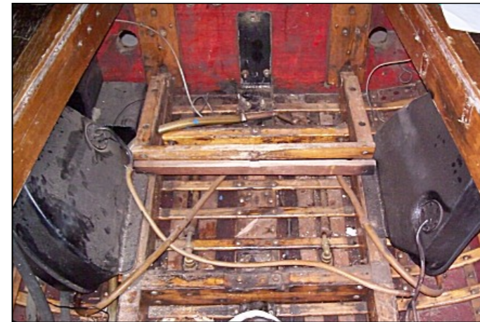
Original dual fuel and oil tanks (the motor is dry sumped). The fuel tanks were modified car tanks and had rusted through the bottom from sitting for 20 years
