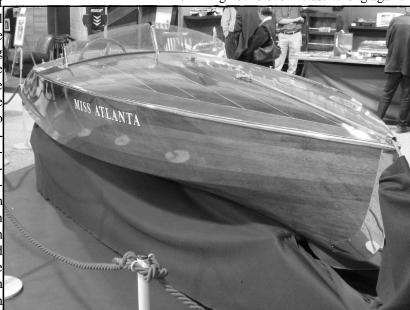
"Miss Atlanta", a superb cravel hulled runabout powered by a very original 100HP Mercury outboard
