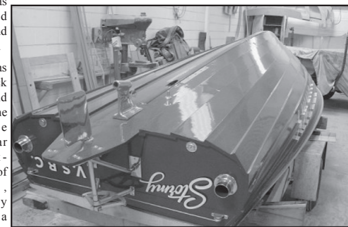
Bottom complete and ready to turn over
