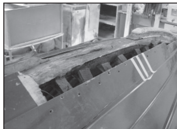
Repairs to the keel area well underway
