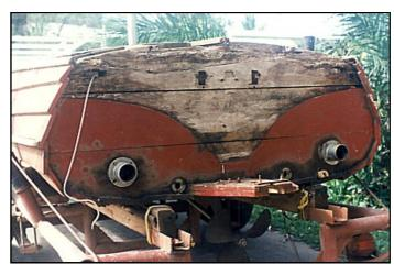
Glenn has been busy since July. The hull has been stripped down and the paint removed. Two lower planks have been repaired and two lengths of planking on the sides were replaced because of some
