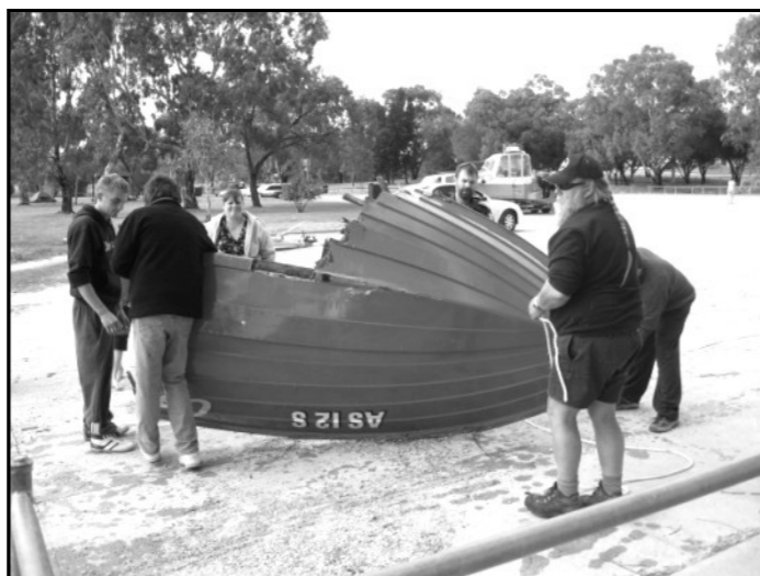
The bow section broke away when pulling the boat up
