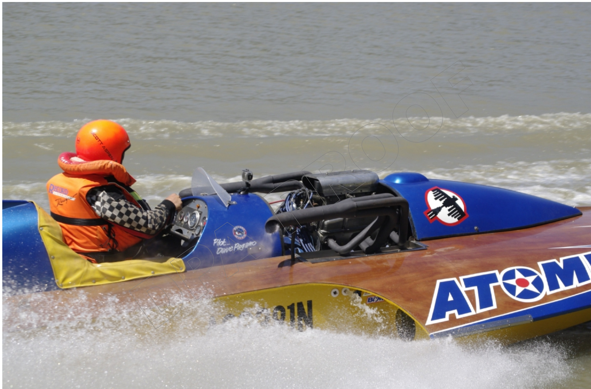
ATOMIC, 1958 17' 6" Jones hydroplane, Holden 308 ci V8
